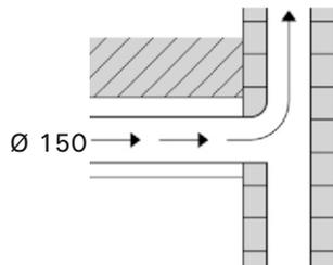
PLEASE NOTE THIS HOOD MUST BE INSTALLED ON MINIMUM 6" ROUND DUCTING OR RECTANGULAR EQUIVALENT
